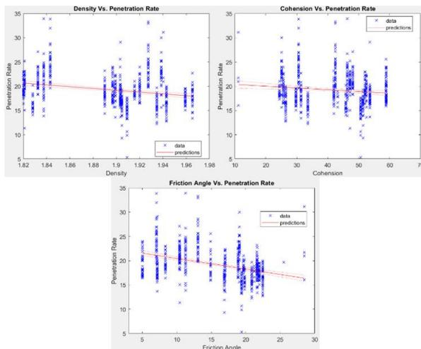
Fig. 5. Upper right: the amount of friction angle changes with penetration rate; Top left: the amount of adhesion changes with penetration rate; Bottom: rate of density changes with penetration rate
