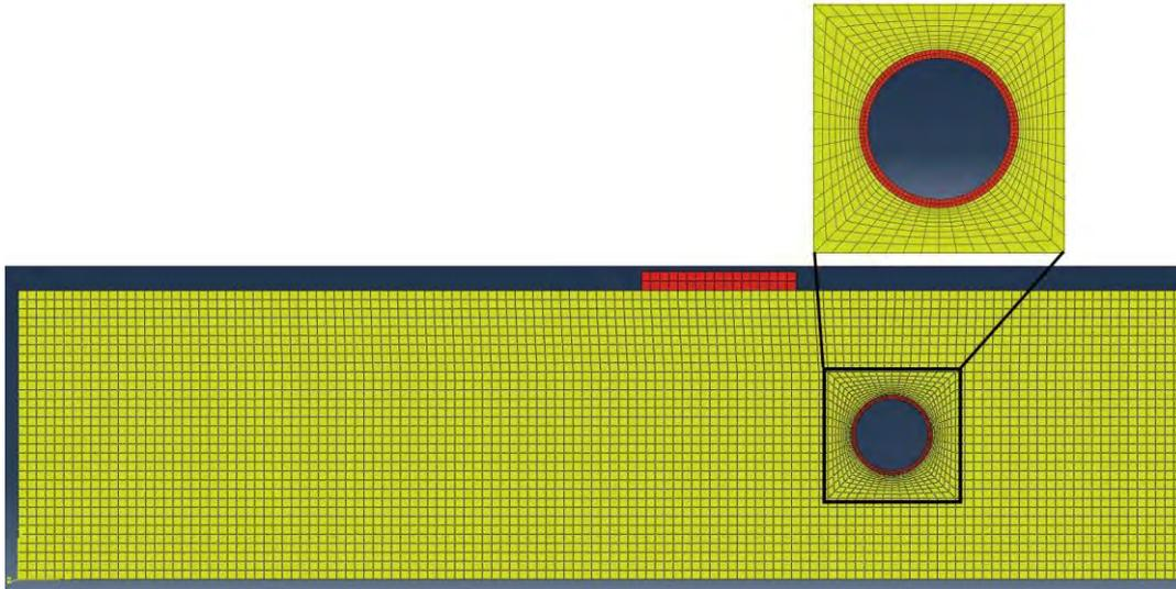
Figure 2. Finite element meshes in the present numerical model
