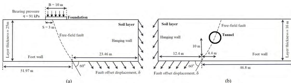
Figure 3. Schematic image of the tests: a) the shallow foundation and fault rupture (after Bransby et al., 2008); b) the tunnel and fault rupture model (after Nabizadeh et al., 2014)
