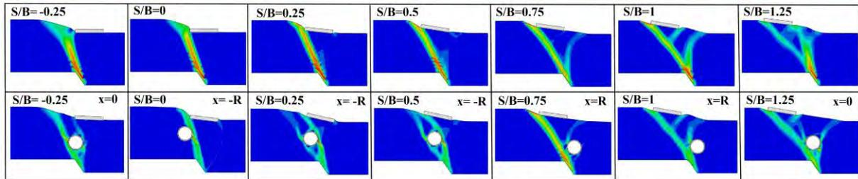
Figure 7. The effect of the presence of a tunnel with internal diameter of  $D = 4\text{ m}$ , embedded in depth of  $y = 8\text{ m}$ , on normal fault–foundation interaction (FE computed plastic strain contours) at  $h = 4\text{ m}$ .
