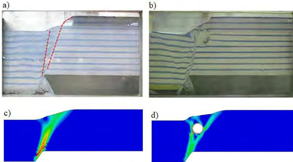
Figure 5. Comparison between experimental results (Nabizadeh et al., 2014) and numerical simulation: a) Deformed soil for the free-field centrifuge test; b) Centrifuge model for the test with tunnel; c, d) Deformed mesh with plain strain contours in finite element analysis
