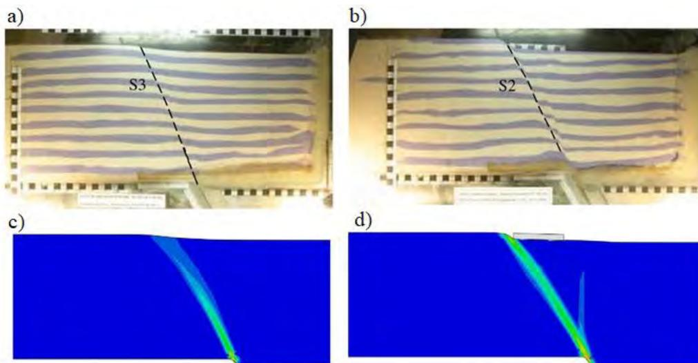
Figure 4. Comparison between experimental results (Bransby et al., 2008) and numerical simulation: a) Deformed soil for the free-field centrifuge test; b) Centrifuge model for the test with foundation ( $S/B=0.3$ ,  $q=91\text{kPa}$ ); c, d) Deformed mesh with plain strain contours in finite element analysis
