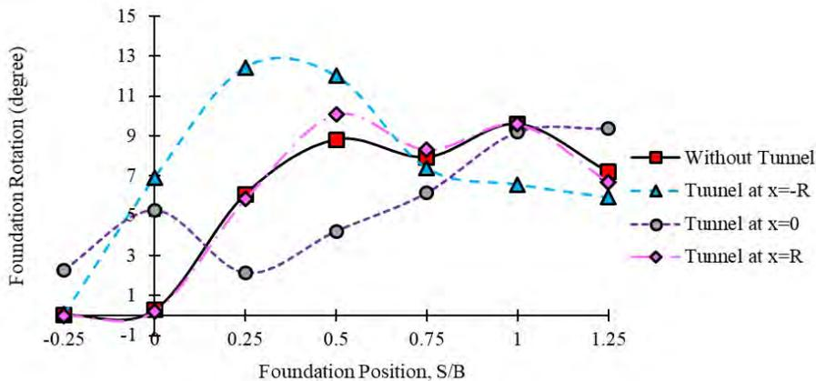
Figure 6. Foundation rotation due to fault rupture.
